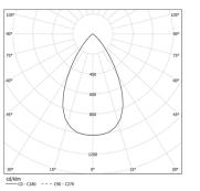
Beam angle Flood 60° Application Weight 0.08Kg
