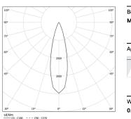
Beam angle Medium 26° Application Weight 0.08Kg
