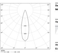
Beam angle Medium 26° Application Weight 0.08Kg
