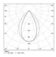
Beam angle Wide flood 76° Application Weight
