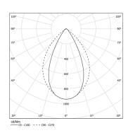
Beam angle Wide flood 76° Application Weight
