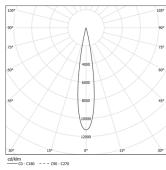
Beam angle Spot 17° Application Weight 2,4Kg
