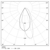
Beam angle Wallwasher Application Weight 2,4Kg
